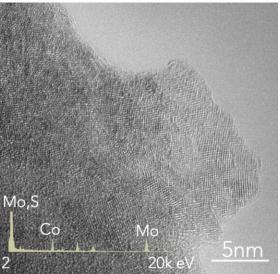
Microscope images show cobalt-doped molybdenum disulfide as grown on a carbon cloth. The high-resolution transmission electron microscope image at right reveals the doped nanosheets, which facilitate the efficient electrochemical catalysis of ammonia. The process was developed for small-scale use by materials scientists at Rice University. Credit: Lou Group/Rice University
