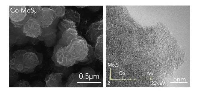
Microscope images show cobalt-doped molybdenum disulfide as grown on a carbon cloth. The high-resolution transmission electron microscope image at right reveals the doped nanosheets, which facilitate the efficient electrochemical catalysis of ammonia. The process was developed for small-scale use by materials scientists at Rice University. Credit: Lou Group/Rice University
