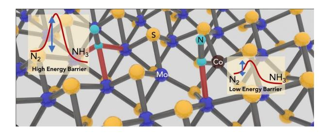
The addition of cobalt atoms to fill vacancies in 2D molybdenum disulfide crystals enhances the material's ability to catalyze ammonia from dinitrogen. Rice University scientists have developed a "green" method for the small-scale synthesis of ammonia that uses less energy and produces less carbon dioxide than industrial processes. Credit: Lou Group/Rice University
