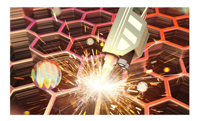
Thermodynamically-efficient, fatigue-resistant elastocaloric cooling materials have been synthesized by additive manufacturing. 3D printing of metals allows versatile shape designs (e.g. a honeycomb structure) of the solid-state refrigerants which also act as heat exchangers in environmentally-friendly cooling systems. Credit: Jiaqi Dai
