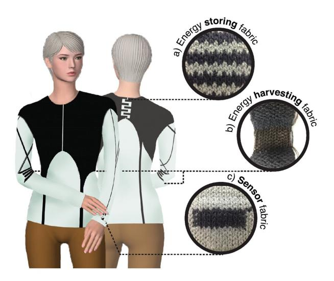
Researchers in Drexel University's College of Engineering and Center for Functional Fabrics have developed a way to coat yarn with conductive MXene materials to make durable functional textiles. Credit: Drexel University
