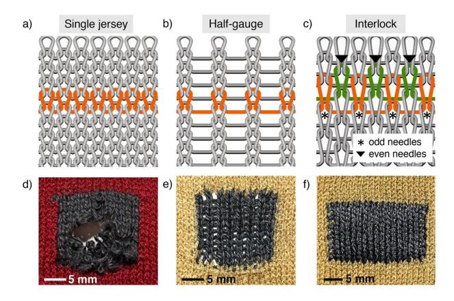
Drexel University researchers developed and tested conductive MXene yarn in industrial digital knitting machines. Credit: Drexel University
