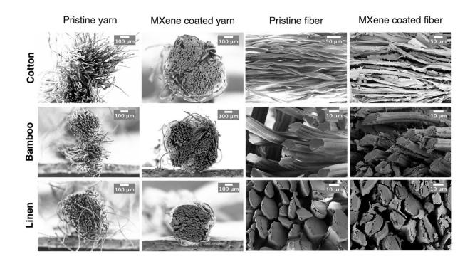
By integrating MXene flakes into the fibers of yarn, researchers at Drexel University can produce functional textiles that are durable enough to wear and wash. Credit: Drexel University
