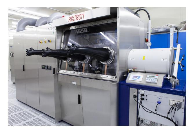
The MOCVD system of Fraunhofer IAF has been modified by the research group to enable the growth of AlScN with sufficient quality and productivity for industry. Credit: Fraunhofer IAF
