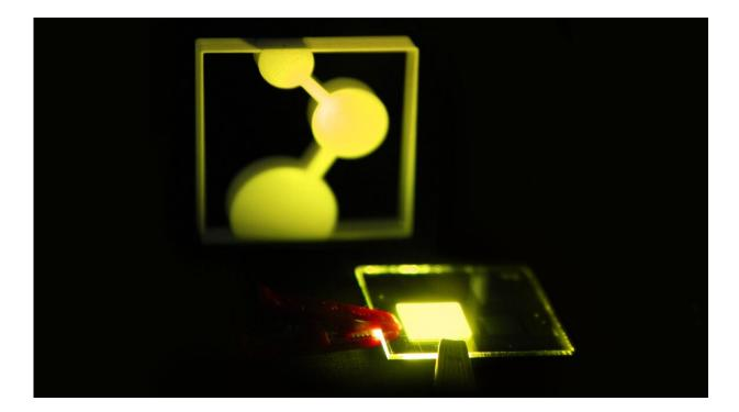
Photograph of the trap-free OLED Credit: MPI-P.
