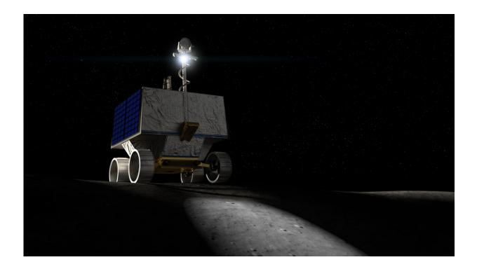
NASA's Volatiles Investigating Polar Exploration Rover, or VIPER, is a mobile robot that will roam around the Moon's south pole looking for water ice. The VIPER mission will give us surface-level detail of where the water is and how much is available for us to use. This will bring us a significant step closer towards NASA's ultimate goal of a sustainable, long-term presence on the Moon – making it possible to eventually explore Mars and beyond. Credit: NASA Ames/Daniel Rutter
