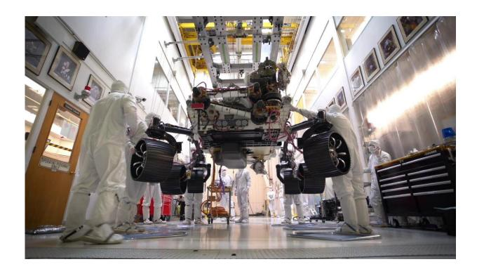
This time-lapse video, taken on Oct. 8, 2019, at NASA's Jet Propulsion Laboratory in Pasadena, California, captures the first time the Mars 2020 rover carries its full weight on its legs and wheels. The rover was photographed in JPL's Simulator Building, where it underwent weeks of testing. Credit: NASA/JPL-Caltech
