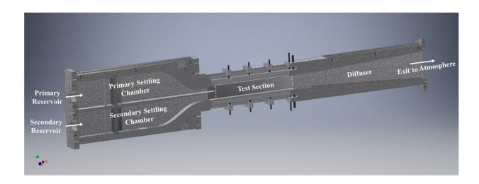
A compressible mixing layer facility CAD schematic. Credit: University of Illinois Department of Aerospace Engineering
