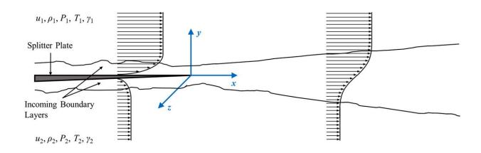
Spatially developing planar free shear layer in laboratory frame of reference. Credit: University of Illinois at Urbana-Champaign
