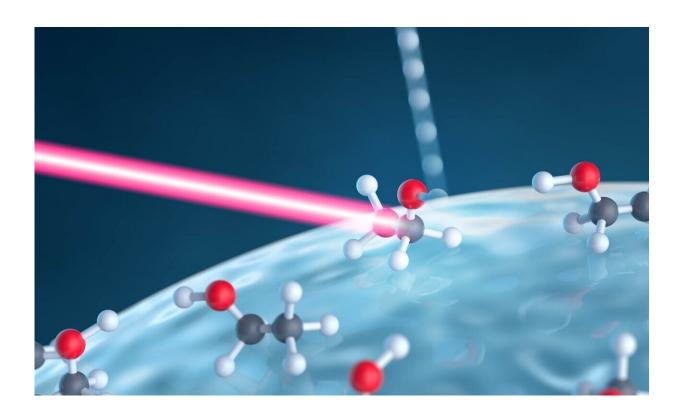
An intense laser pulse (red) hits a nanoparticle made of glass and interacts with molecules on its surface. Subsequently, as depicted, hydrogen ions may be detached, and the yield of such reactions can be measured by reaction nanoscopy. Credit: Alexander Gelin
