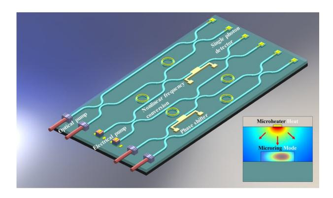
Researchers created the first thermally tunable optical switch using a silicon carbide-on-insulator platform. The schematic image shows their concept for a quantum photonics integrated circuit chip that includes the circular microring resonators and microheaters reported in Optics Letters. The inset shows the temperature and electric field distributions at the cross-section of a microring resonator heated by a microheater. Credit: Ali Adibi, Georgia Institute of Technology
