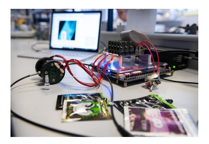
The prototype test takes only five minutes to search for spice in a saliva sample. Credit: University of Bath
