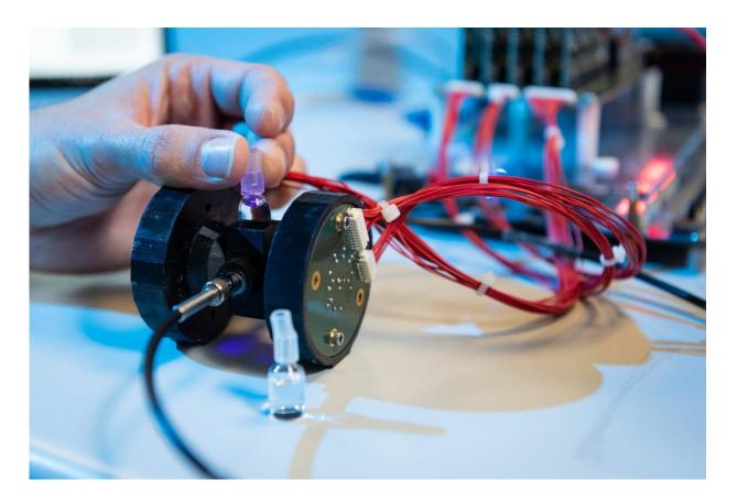
The prototype test takes only five minutes to search for spice in a saliva sample. Credit: University of Bath
