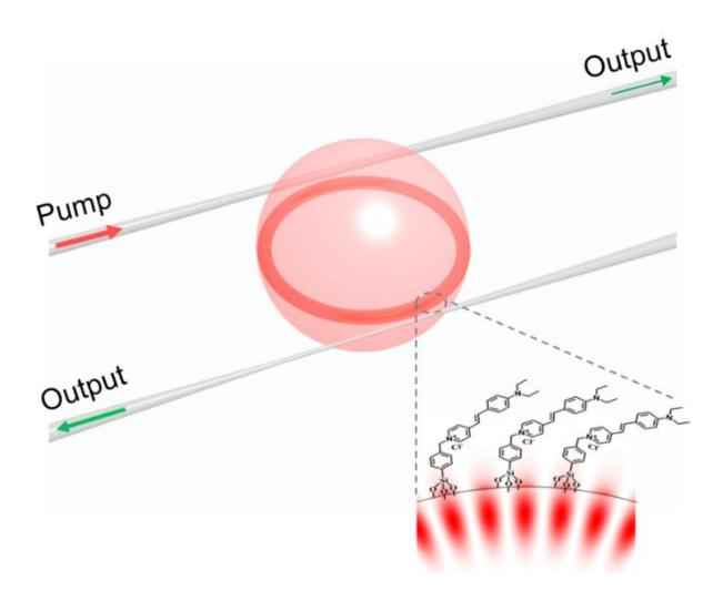
Figure 1: Schematic of the organically functionalized silica microcavity with dual fiber couplers. Credit: Peking University
