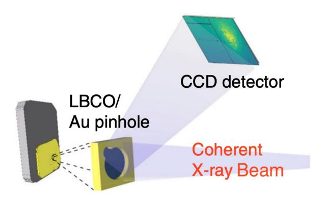
The schematic shows how a speckle pattern is measured: first the coherent x-ray beam delivered by the beamline is focused onto the sample, then the x-rays are scattered by the sample at a specific angle (sensitive to the charge density wave presence)and captured by the CCD detector. The pinhole provides a mask, allowing the researchers to illuminate only a small, specific area of the sample. Credit: Brookhaven National Laboratory
