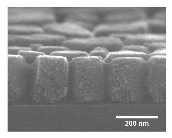
This scanning electron microscopy image clearly shows the 12 nm nanocubes assembled into supercrystals. Credit: Verner Håkonsen/NTNU
