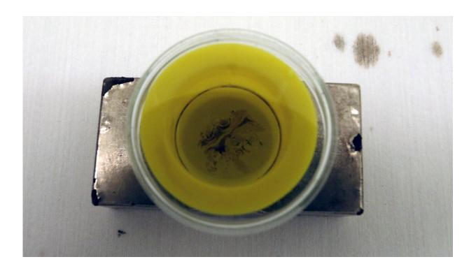
This lab thimble is full of nano-sized supercrystals. The pattern you can see is from the supercrystals arranging themselves. Credit: Nancy Bazilchuk/NTNU
