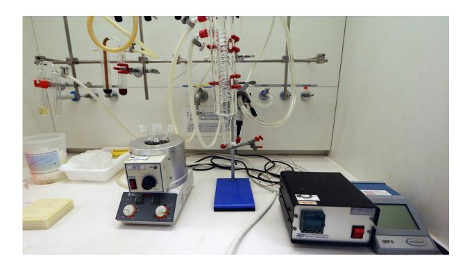
Tools of the trade: a three-necked flask (left) to cook up the solution that makes nanocubes, and a complex piping system that condenses the solution if it evaporates and controls the gas flow during the reaction. Credit: Nancy Bazilchuk/NTNU
