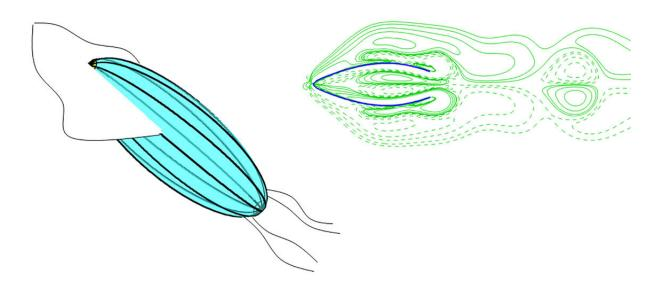
Xiaobo Bi and Qiang Zhu discuss their work developing an aquatic robot inspired by cephalopods. (Left) Envisioned squid-inspired robot that combines fin flapping and jetting for locomotion. (Right) Numerical simulations provide insights of the underlying physical mechanisms. Credit: Qiang Zhu
