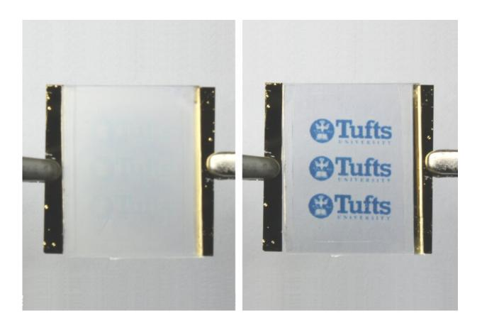
Passing a voltage across a heating element connected to the silk bilayer expands the material and erases the wrinkle pattern (left). Cutting off voltage allows material to cool and the wrinkle pattern appears (right). Credit: Fio Omenetto, Tufts University
