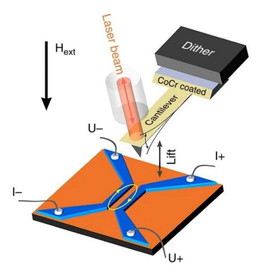
Experimental setup. The blue and orange indicate niobium and copper, respectively. The ellipse marks the area of the Josephson junction. The cobalt-chromium-coated tip oscillates, excited by a piezo element (dither). The optic fiber is used to read out the oscillations. Credit: Viacheslav Dremov et al./Nature Communications
