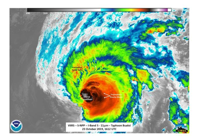
NASA-NOAA's Suomi NPP satellite passed over Typhoon Bualoi and the VIIRS instrument aboard captured this image of the storm on Oct. 23, 2019 at 12:12 p.m. EDT (1612 UTC). Suomi NPP found that the strongest thunderstorms west of center had cloud top temperatures as cold as 190 Kelvin (minus 117 degrees Fahrenheit/minus 83.1 Celsius). Credit: NASA/NOAA/UWM-CIMSS, William Straka III
