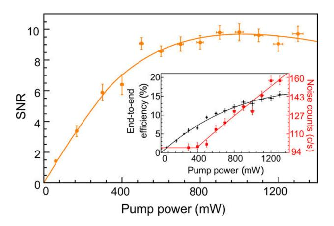
Signal-to-noise-ratio (SNR) measured after filtering of the frequency-converted ion signal. The orange curve is the SNR given the measured conversion efficiencies and noise at each pump power. Inset: Measured conversion efficiency (black) and measured noise counts (red) on the APD as a function of pump power. The black curve is a theoretical fit to the efficiency data, and the red curve is an empirical fit to the noise. Credit: Science Advances, doi: 10.1126/sciadv.aav4651
