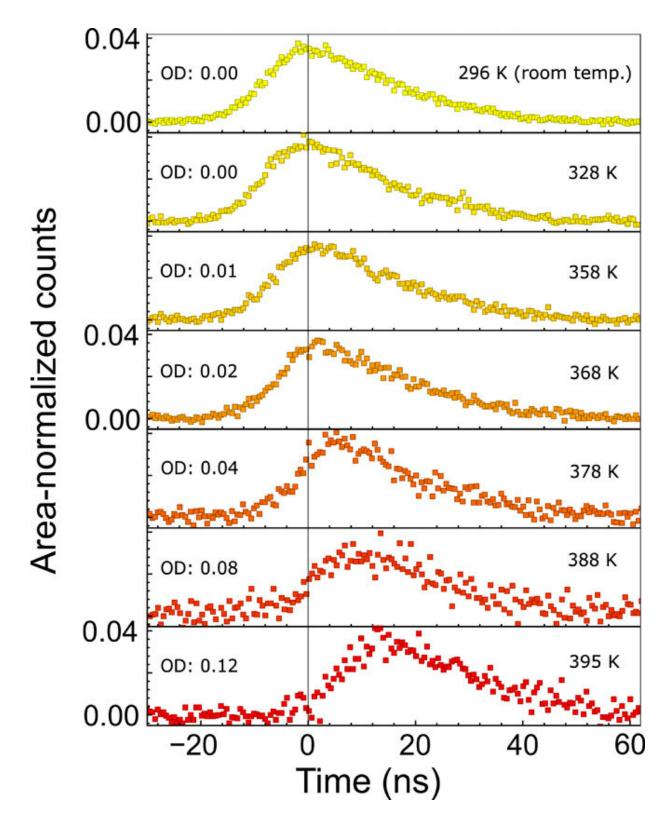
Area-normalized temporal photon shapes. Area-normalized temporal shapes of frequency-converted photons that have passed through a warm 87Rb vapor cell.
