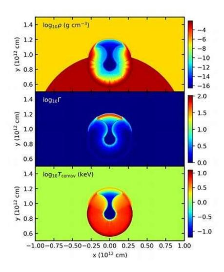
Spatial distributions of matter density (top), Lorentz factor (middle) and comoving temperature (bottom) at t = 11 s, showing the mildly relativistic reflection wave propagating backward in the cavity, as well as the ultrarelativistic electron positron plasma wave propagating outside the cavity. The shock wave is
