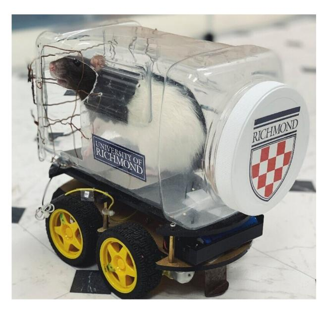
Scientists modified a robot car kit by adding a clear plastic food container to form a driver compartment with an aluminum plate placed on the bottom
