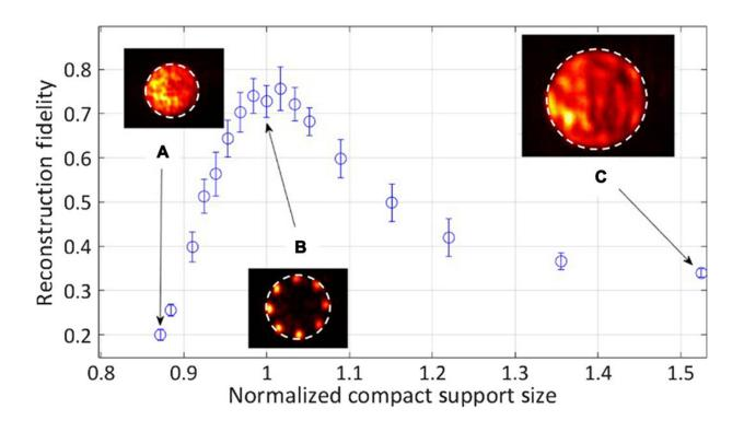
Experimental quantitative results for reconstruction fidelity as a function of the compact support radius of the aperture normalized by the object size. Insets: Typical reconstructed object intensity distributions. (A) Compact support radius
