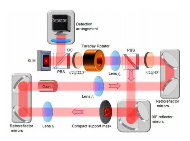
Detailed experimental digital ring degenerate cavity laser arrangement. SLM - spatial light modulator; PBS - polarizing beam splitter;  $\lambda/2@22.5^{\circ}$  - half-wave plate at 22.5° angular orientation;  $\lambda/2@45^{\circ}$  - half-wave plate at 45° angular orientation; compact support mask - intra-cavity aperture at the Fourier plane; OC–output coupler. Credit: Science Advances, doi: 10.1126/sciadv.aax4530
