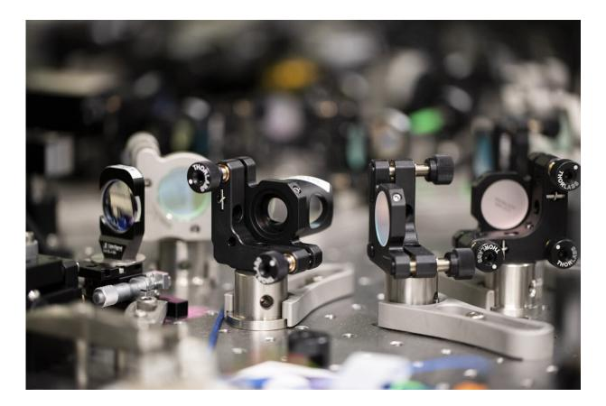
A network of optical devices -- mirrors, beamsplitters, and optical fibres -- weave laser light into an optical quantum processor. Credit: CQC2T
