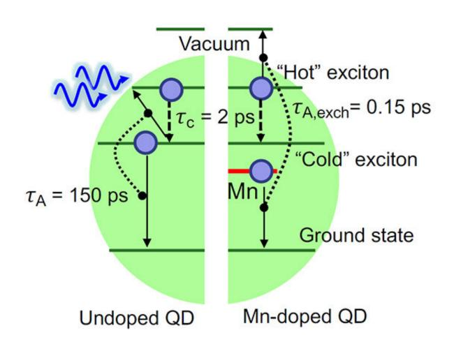
Doping a quantum dot with manganese (right half of graphic) speeds the capture of energy from a hot electron to 0.15 picoseconds, outpacing losses to phonons in the crystal lattice. Credit: Los Alamos National Laboratory
