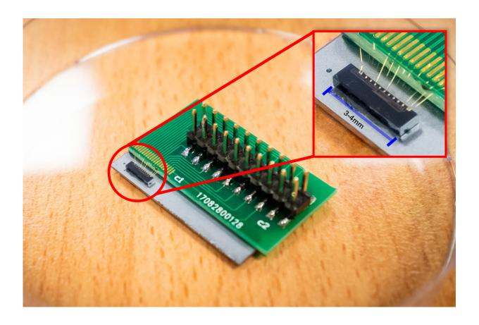
Roughly about 3mm in size, tiny chip developed by NTU scientists uses quantum communication algorithms to provide enhanced security compared to existing industry standards. It also needs 1,000 times less space than current quantum communication setups, opening doors for more secure communication technologies that can be deployed in compact devices such as smartphones, tablets and smart watches. Credit: NTU Singapore
