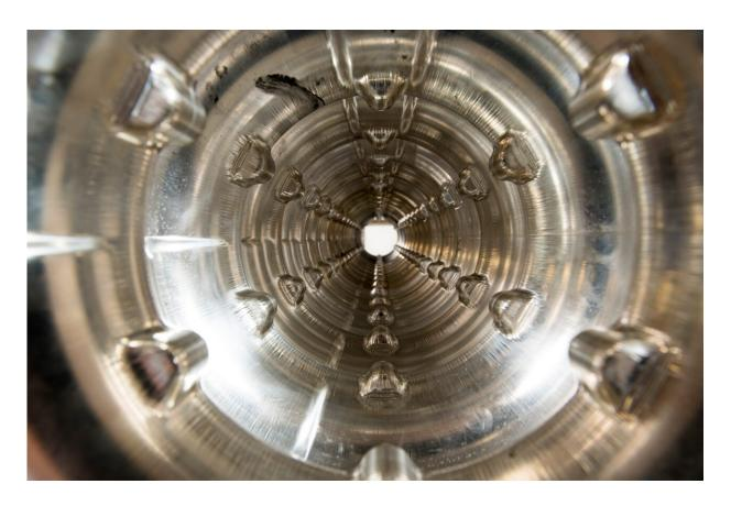
This shows a view down the center of the magnet module. Credit: Reidar Hahn, Fermilab
