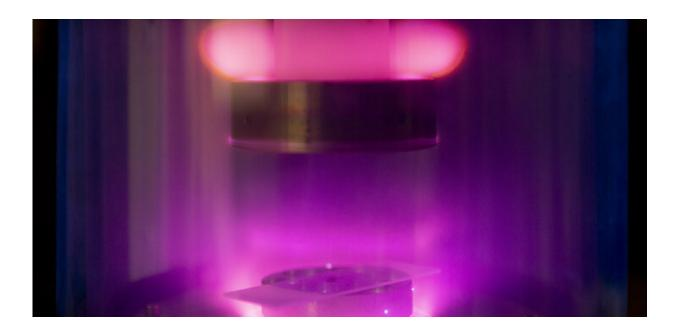
This air-plasma (the violet-blue glow) facility was used to treat the sample grids used in electron microscopy. Credit: KAUST
