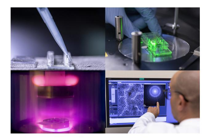
These images capture stages of the sample preparations performed for singlemolecule fluorescence and cryo-TEM microscopy. Rachid Sougrat of the Imaging and Characterization Core Lab helps to analyze the results (bottom right). Credit: KAUST
