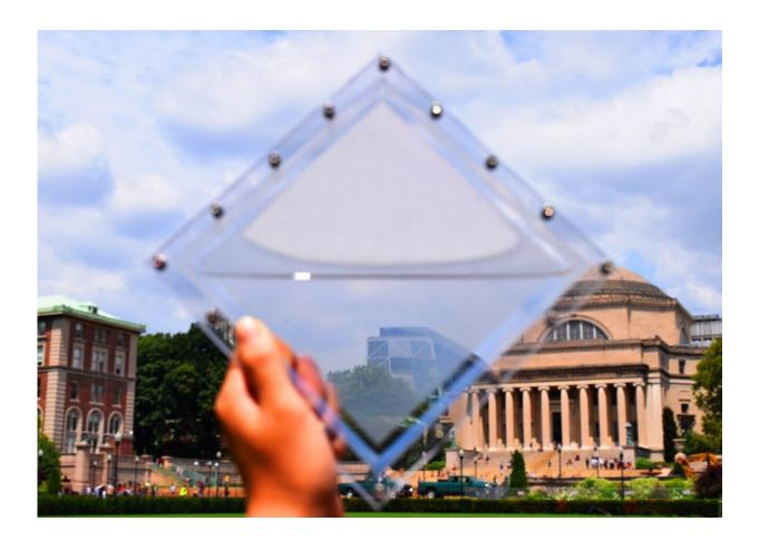
The porous polymer coatings, which switch from white to transparent when wetted, can be put into plastic enclosures to make panels that control light and temperatures of buildings. Credit: Jyotirmoy Mandal/Columbia Engineering
