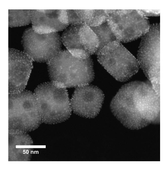
Electron micrograph of the platinum nanoparticles distributed onto perovskite
