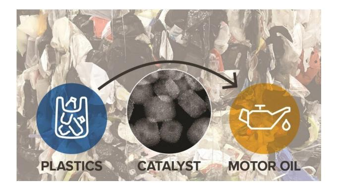
The catalyst of platinum nanoparticle/perovskite nanocuboid transforms discarded plastics into a higher value product (for example, motor oil). Credit: Argonne National Laboratory
