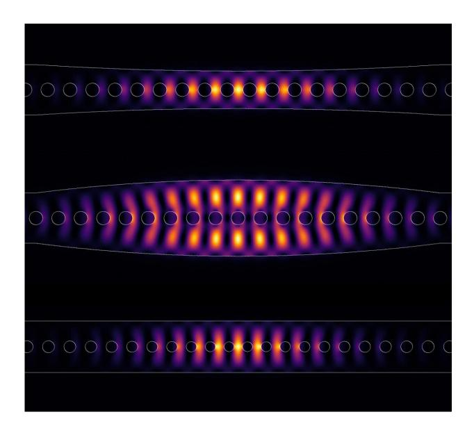
Various designs form photonic crystals which concentrate light in a cavity. Credit: J. Olthaus, P. Schrinner et al./Adv. Quantum Technol.
