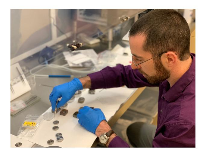
Evan Groopman, a research physicist, prepares a microscopic uranium particle sample to be measured in the NAUTILUS instrument in the Accelerator Mass Spectrometry Laboratory at the U.S. Naval Research Laboratory in Washington, D.C., Sept. 5. Credit: U.S. Navy photo by Nicholas E. M. Pasquini
