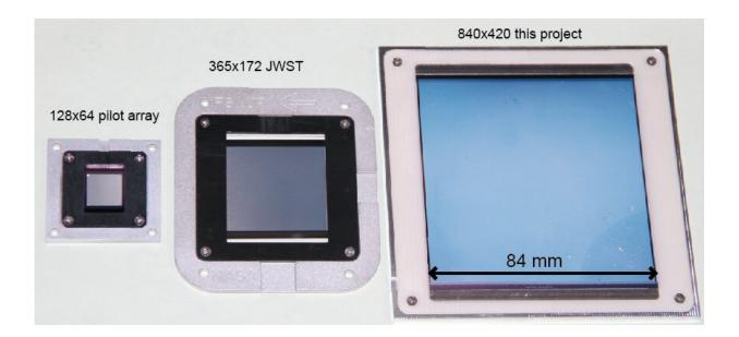
The Goddard-developed microshutter array technology has evolved since its initial development in the 1990s for the James Webb Space Telescope. Here are images of its various incarnations. A Next-Generation Microshutter Array will fly in space for the first time on October 27, 2019. Credit: NASA
