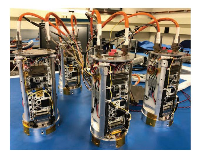
A team of Wallops Flight Facility engineers will release these instrumented subpayloads to demonstrate the distributed payload communications technology. The devices should collect and transmit about four minutes of data before reentering the atmosphere. Credit: NASA/Scott Hesh
