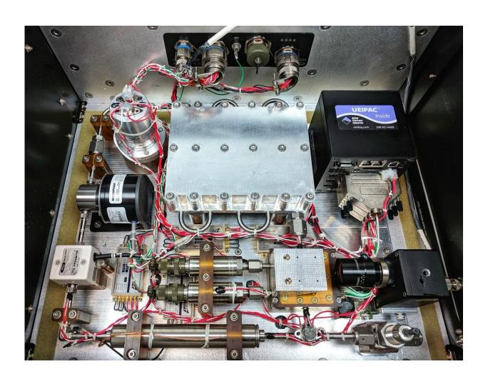
The microgap-cooling technology developed by Goddard technologist Franklin Robinson and University of Maryland professor Avram Bar-Cohen was tested twice on a Blue Origin New Shepard rocket. Credit: NASA/Franklin Robinson
