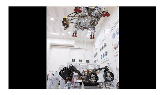
In this picture from Sept. 28, 2019, engineers and technicians working on the Mars 2020 spacecraft at NASA's Jet Propulsion Laboratory in Pasadena, California, look on as a crane lifts the rocket-powered descent stage away from the rover after a test. Credit: NASA/JPL-Caltech
