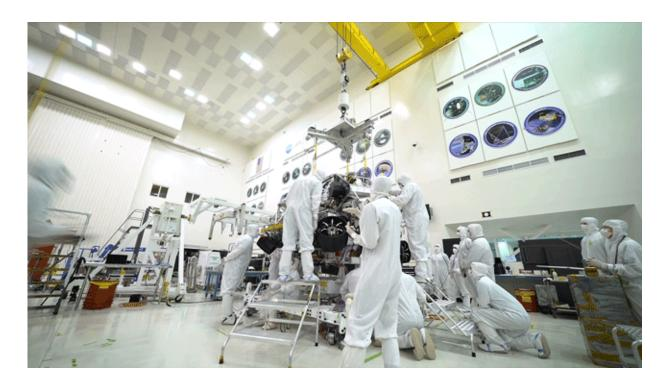
Time-lapse animated gif of engineers and technicians working on the Mars 2020 spacecraft, look on as a crane lifts the rocket-powered descent stage away from the rover. Credit: NASA/JPL-Caltech
