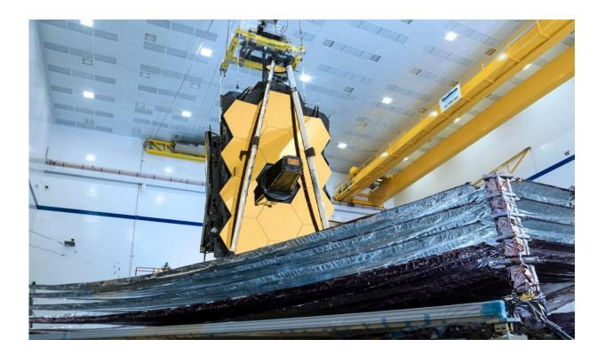
NASA's James Webb Space Telescope is seen with its revolutionary five-layer sunshield fully deployed, standing tall in Northrop Grumman's clean room in Redondo Beach, California. Credit: NASA/Chris Gunn
