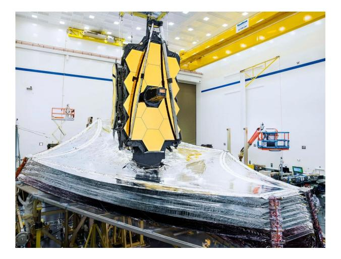
After successfully assembling the entire observatory, technicians and engineers moved on to fully deploy and tension all five layers of its tennis court sized sunshield, which is designed to keep its optics and sensors in the shade and away from interference. Credit: NASA/Chris Gunn
