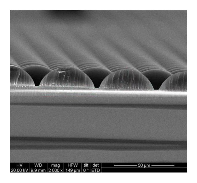
A close up of the film which combines nanocrystals and microlenses to capture infrared light and convert it to solar energy. Credit: KTH Royal Institute of
