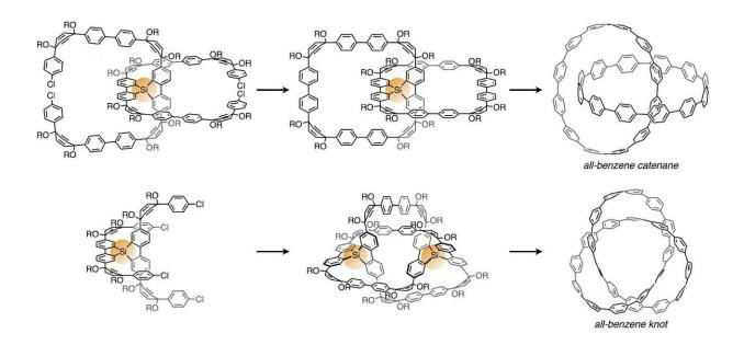
Synthesis route of an all-benzene catenane (top) and knot (details). First, the chlorine atoms (Cl) parts were reacted through a reaction with nickel to form carbon-carbon bonds. After that, the silicon atoms were removed by using fluorine, and then the crimped parts (OR) were removed through a reaction with sodium to convert into benzene rings. Credit: Nogoya University
