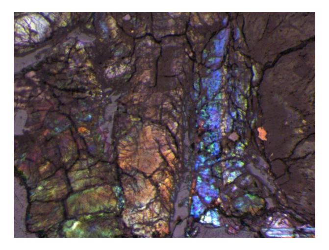
Magnified view of a meteorite specimen from Mars under cross-polarized light. Image taken with UD's new atomic force-Raman microscope. Credit: University of Delaware
