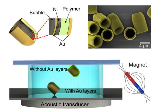
A schematic showing the structure the microrockets, which are 3D printed and contain a trapped air bubble (top left), and how they look under scanning electron microscopy (top right). The acoustic fluidic chamber where they can be driven in three dimensions is shown on the bottom. Credit: Liqiang Ren
