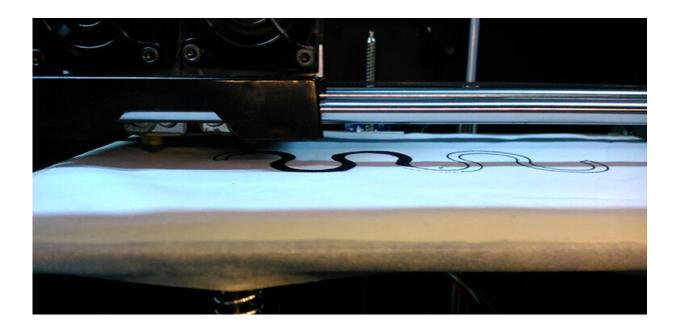
A polymeric material with electrically conductive properties is 3-D-printed directly on the textile (thesis cover photo). Credit: University of Borås
