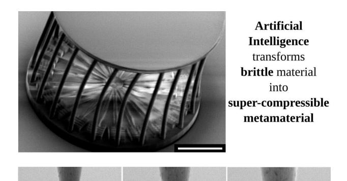
Metamaterial created with Artificial Intelligence that transforms a brittle material into a sponge-like material. Unlike a sponge, this metamaterial is stiff until a critical force is reached after which it becomes easily compressible. Credit: Delft University of Technology
