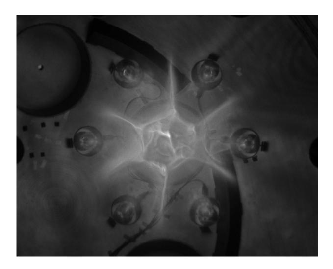
Supersonic jets fired from 7 plasma guns collide in PLX test firings. In addition to debugging the machine, the experiments provide data to verify models of colliding plasmas important for astrophysics, aeronautics, and various controlled fusion schemes. Credit: Los Alamos National Laboratory
