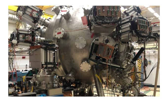
Half of the 36 supersonic plasma jets that will make up the Plasma Liner Experiment at Los Alamos National Laboratory have been installed. The remaining jets will be added and fully spherical plasma liner experiments will commence by the end of 2020. Credit: Los Alamos National Laboratory
