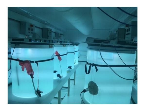
Tanks (300-L 'minicosms') in which onboard experiments will be performed during the TONGA Project. Each tank will contain different mixtures of surface waters and hydrothermal fluids, to simulate the fertilising or toxic effects these fluids have on biological communities, and especially on phytoplankton. Credit: C. Guieu
