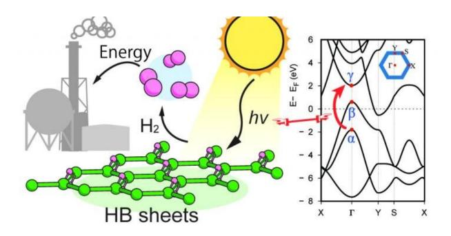
The hydrogen storage and release capacity of HB sheets is exceptionally high due to their two-dimensional nature and unique electronic band structure. Credit: Nature Communications
