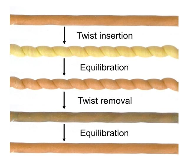
This natural rubber fiber has been coated with a paint that changes color when the fiber changes temperature. University of Texas at Dallas researchers and their colleagues in China recently showed that when the rubber fiber is twisted, it
