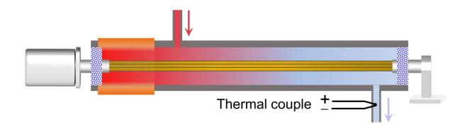
The device for cooling flowing water by twist release of nickel titanium wires or rubber fibers. Credit: University of Texas at Dallas
