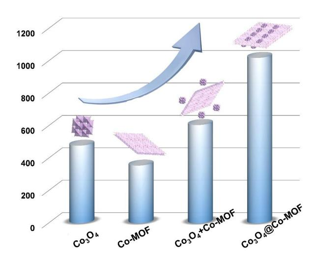
A bar graph for capacitance performance comparison of electrode materials. Credit: ©Science China Press
