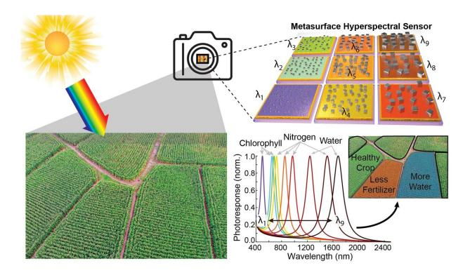
A new type of lightweight, inexpensive hyperspectral camera could enable precision agriculture. This graphic shows how different pixels can be tuned to specific frequencies of light that indicate the various needs of a crop field. Credit: Maiken Mikkelsen and Jon Stewart, Duke University
