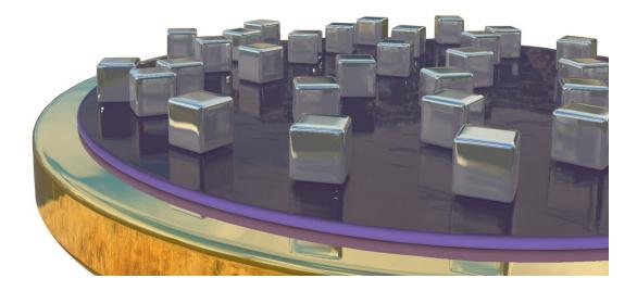
Artistic rendering of a new type of hyperspectral imaging detector. Depending on their size and spacing, nanocubes sitting on top of a thin layer of gold trap specific frequencies of light, which heats up the materials beneath to create an electronic signal. Credit: Jon Stewart, Duke University
