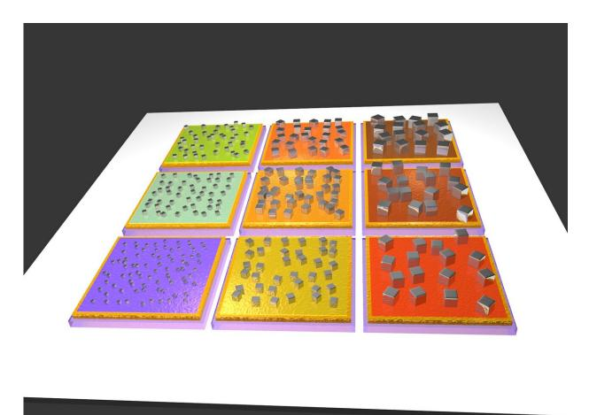
The new hyperspectral imaging device relies on a 'mega-pixel' consisting of a grid of smaller pixels, each tuned to a different frequency of light by controlling the size and spacing of the nanocubes sitting on their surfaces. Credit: Jon Stewart, Duke University
