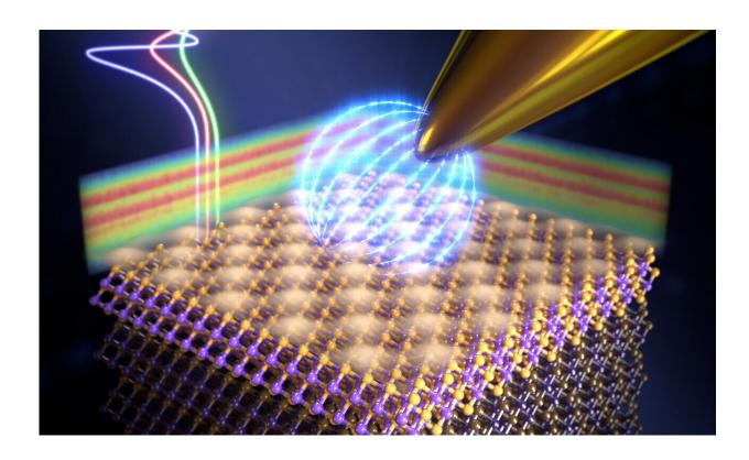
The gold tip is moved across the surface of the topological insulator and experiences energy loss only at discrete, quantized energies. This is related to the image potential states that are formed over the conducting surface of the topological insulator. Credit: University of Basel, Departement of Physics
