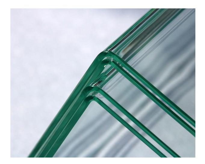
Using the new laser-based glass-bending process, it is possible to achieve precisely defined and extremely small bend radii, so that even laminated safety glass can be bent around a corner. The sheets of glass in the image are three
