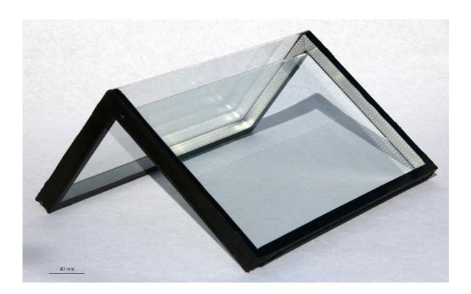
A double-glazed corner element produced with the new glass-bending process. Credit: Fraunhofer IWM
